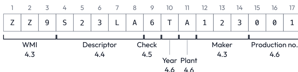
Figure 1 — Structure of the vehicle identifier, with the example of Annex A (illustrative; ZZ9 is not an assigned WMI)
